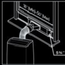
Horizontal Duct Installation :
