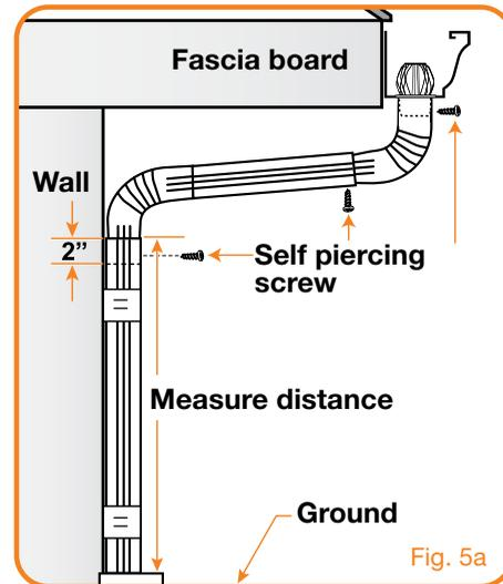
On the ground, cut or add downpipe sections together as required. To join downpipe sections together screw as illustrated.
