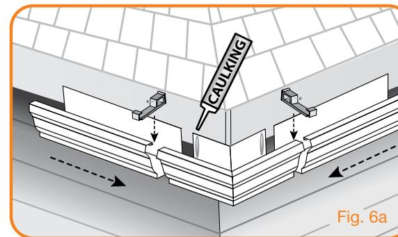
Add gutter sealant to seams of box mitre to ensure it is water tight (Fig. 6b)
