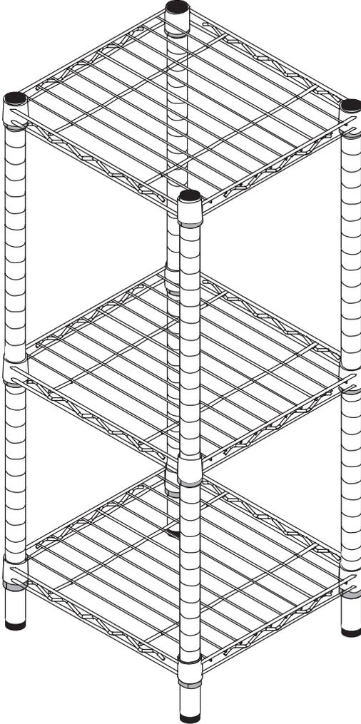
1. Use leveler feet to adjust legs when shelf is on an uneven surface.
