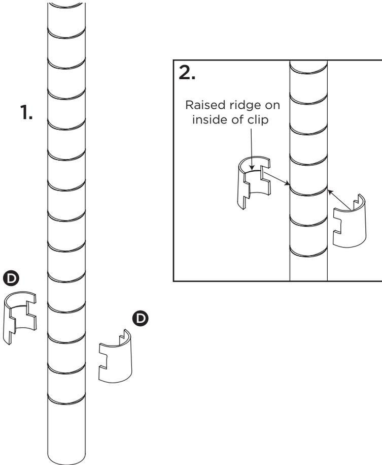
1. The shelves (A) are held on with pairs of the shelf support clips (D). Align two halves of the shelf support clips (D) on the support pole at the desired height of the bottom shelf. \*\*\*When clips are together they form a slight cone shape. The top of the clips is the thin end.\*\*\*
