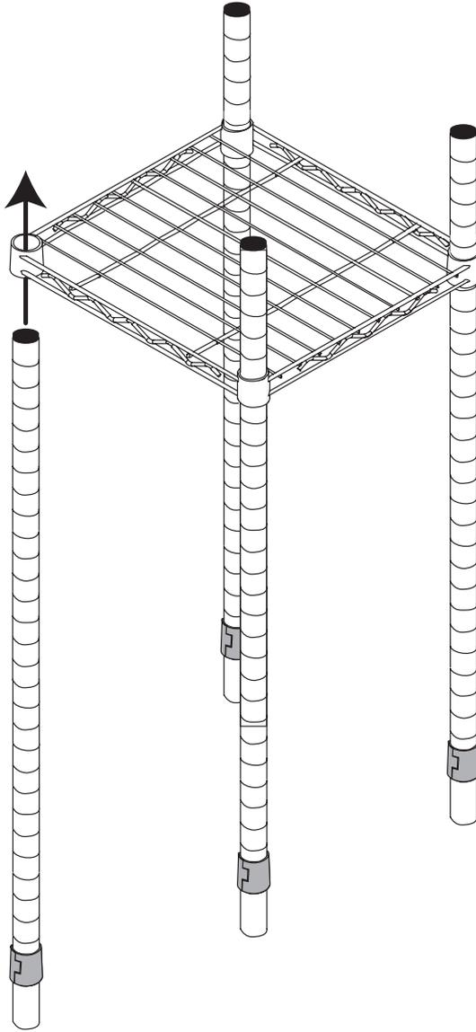
1. Slide all four poles through shelf. Once you have verified that all support clips are aligned push shelf firmly down until snug.
