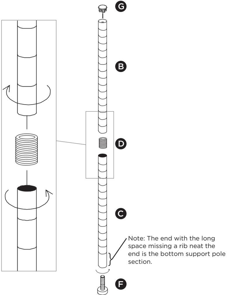
1. Begin by identifying the top and bottom of pole support sections (B & C) see illustration above.
